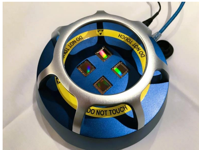
Figure 2: Image of the PFO1040 monitor developed for terrestrial applications utilising four imaging sensors and incorporating an illumination ring
